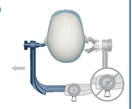
Pull with small force in the **opposite direction** to make sure that the release knob is secured.
