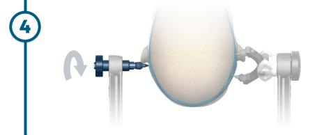
Increase the pin force by means of the **torque screw**.
