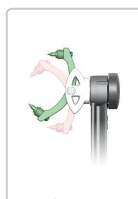
If vertically aligned, arrange the two-pin-holder directed upwards.
